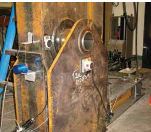
Figure 20. Close-up view of the Pin-Fuse structural solution under testing. © Skidmore, Owings & Merrill LLP
