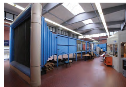
Figure 7. A view of the CRIACIV Atmospheric Boundary Layer Wind Tunnel from the inlet.
