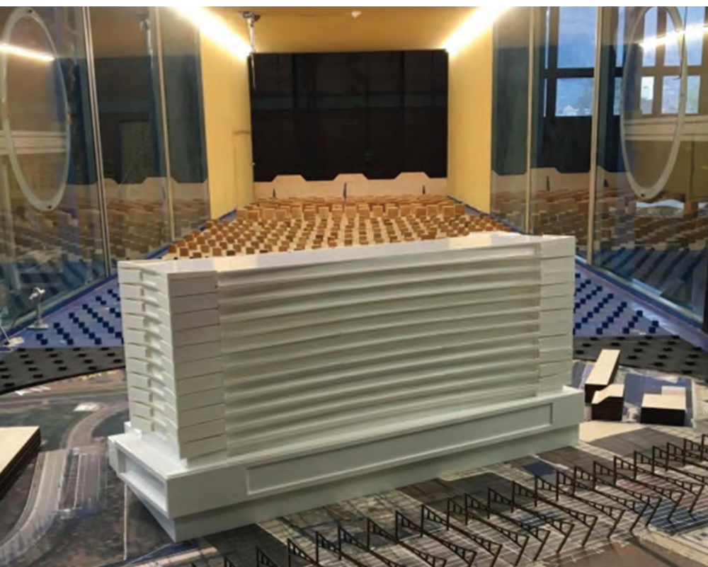
Figure 4. A scale model of a tall building with a complex façade inside the CRIACIV wind tunnel. View is from inside the wind tunnel towards the inlet.
