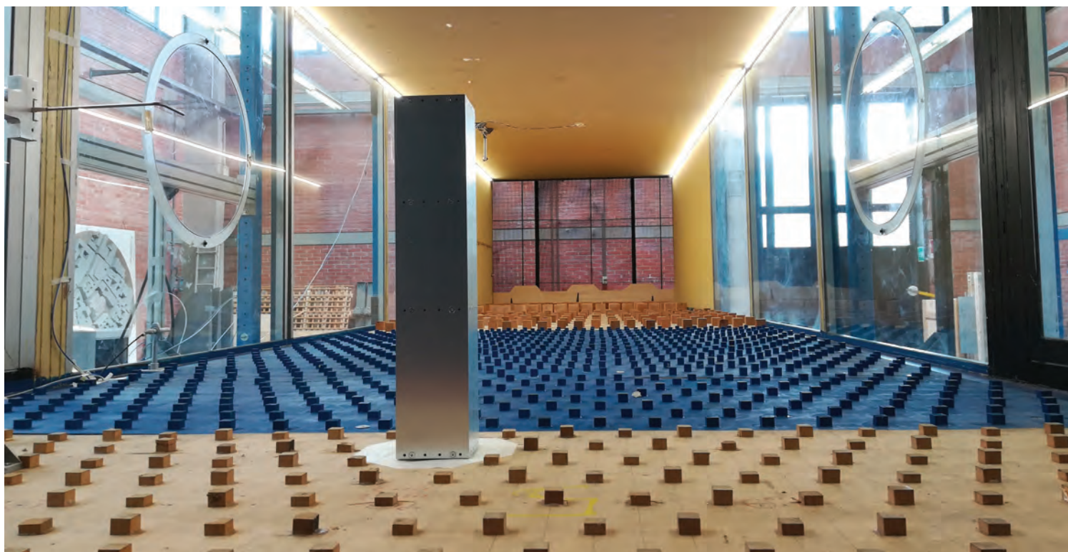
Figure 8. A picture inside the CRIACIV wind tunnel, facing from the working section to the inlet, showing the set-up needed to reproduce the Atmospheric Boundary Layer (ABL).
