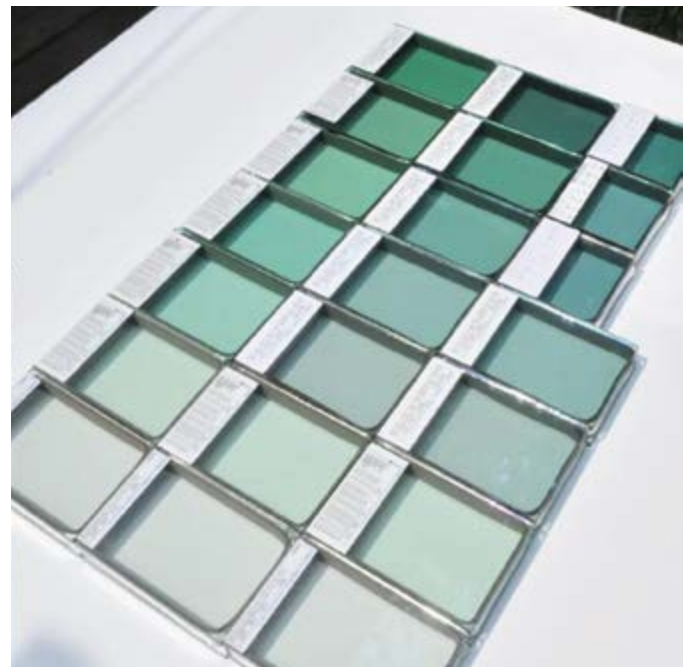
Figure 11. Through innovative coating-on-demand technology, the building's glass was able to be completely customized for both performance and color gradient. The project team tested numerous iterations of the glass as it came out of the manufacturing line.
