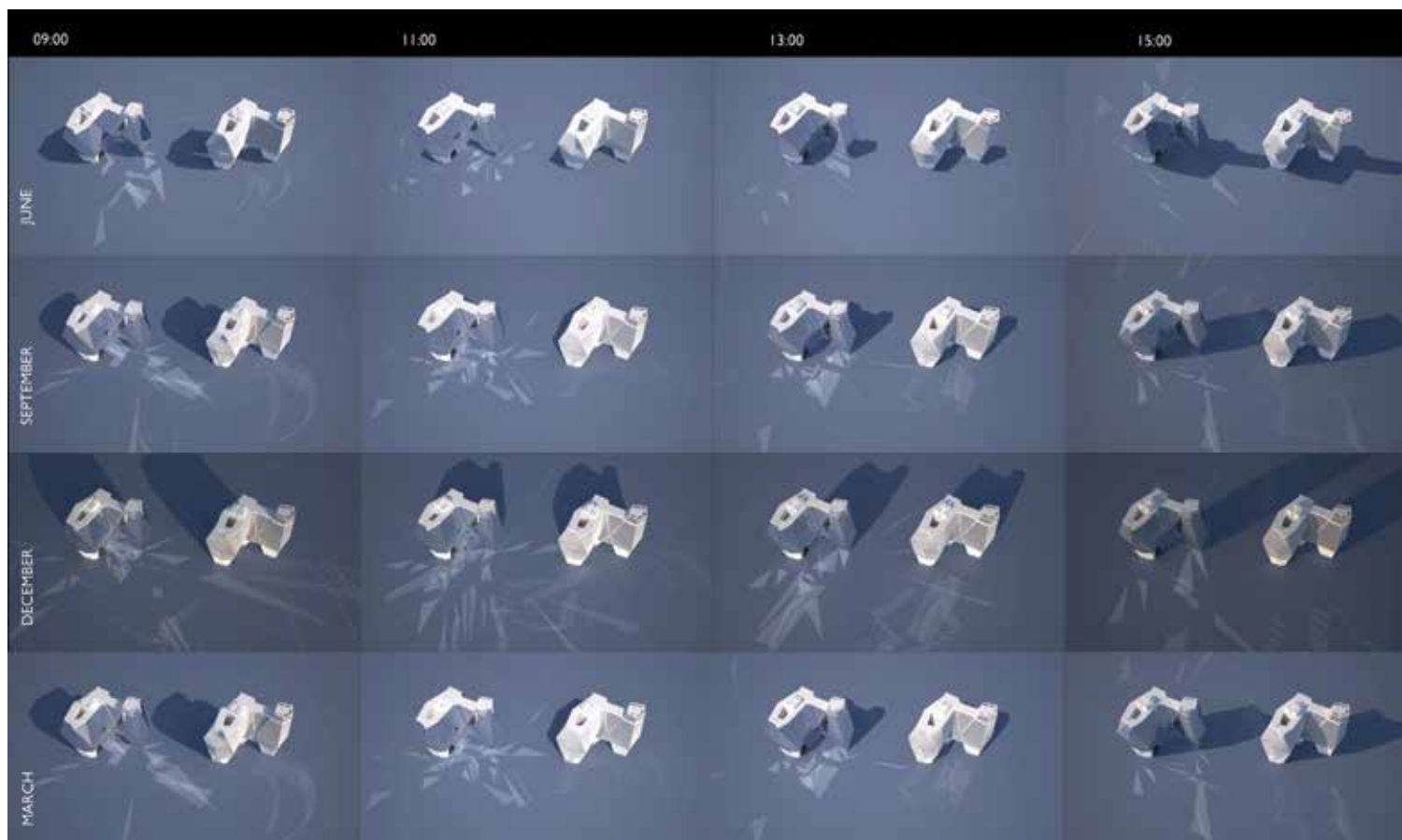
Figure 10. Reflectivity and shading analysis. © Ron Arad Architects
