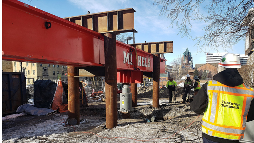
Figure 10. Pile Static Load Testing. (© Thornton Tomasetti)
