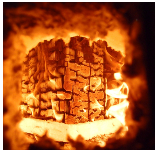
Figure 13. 3-Hour Fire Test. (courtesy of Korb + Associates)
