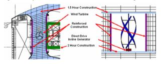
Figure 1 - Wind Turbine Layout and Protection Strategy
