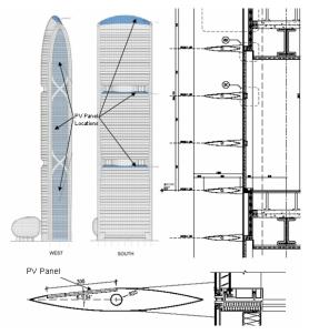
Figure 2 - Photovoltaic Panel Locations and Building Integration
