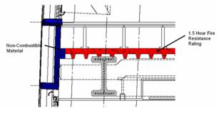
Figure 3 - Typical Fire-resistant Joint System at Double Curtain Wall
