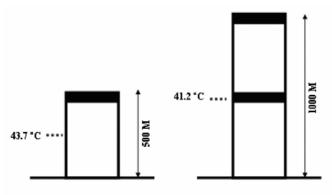
Figure 3: ADLR Lapse Rate Temperature at the Middle Floor of a 500 M (1640') Tall vs. 1000 M (3,280') Tall Building
