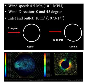
Figure 9: CFD Modeling of Wind Driven Ventilation; Left: Aligning a 10 M<sup>2</sup> (107.6 Ft<sup>2) Opening</sup> with Prevailing Wing; Right: Turning the Opening 45 Degree Away from Prevailing Wind (SOM LLP)
