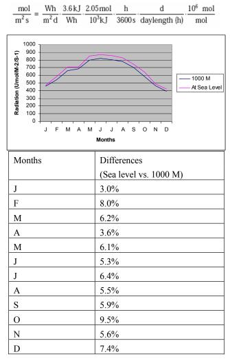
Figure 11: Solar Radiation Differences between Sea Level and 1 kM (3,280 Ft) using Regression Analysis on Measured Data (SOM LLP)
