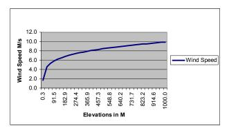
Figure 8: Wind Speed Changes of a 1 kM (3,280 Ft) Tower in Dubai (SOM LLP)
