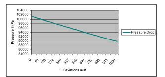
Figure 6: Air Pressure Change for a 1 kM (3,280 Ft) Tower in Dubai (SOM LLP)
