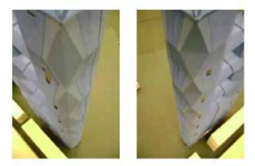
Figure 6. Istanbul Tower: twin tower corner variations (Source: BMT Fluid Mechanics / Buro Happold) 图6. 伊斯兰布尔大厦:连体塔楼的楼角变化(资料来源: BMT Fluid Mechanics / Buro Happold)
