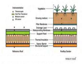
Figure 3: Typical components of normal roof and rooftop garden (Liu, 2002)
