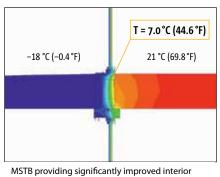
MSTB providing significantly improved interior surface temperatures
