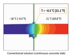
Figure 5. Thermal profile of the three connection details.
