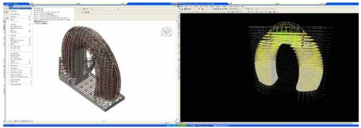
Figure 3. BIM model and structure analysis model two-way interaction 图3. BIM模型与结构分析模型双向联动
