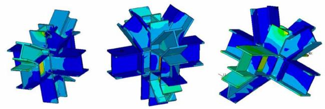
Figure 4. stress map of the detail connection 图4. 节点应力云图
