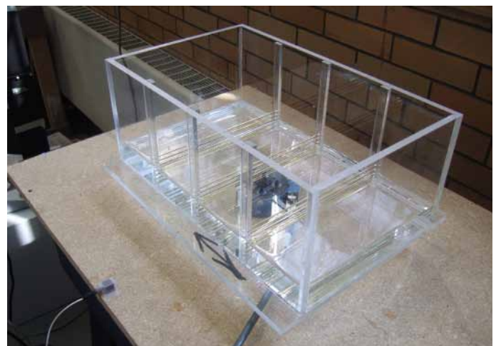
Figure 7. Experimental setup for a combined structure-TSD system in the HIL simulation (Source: Dae Kun Kwon)
