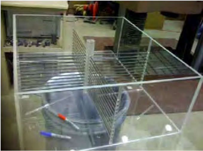
Figure 3. Tuned sloshing damper model (scale 1:10) (Source: Ahsan Kareem and Deepak Kumar) 图3. 可调谐液体晃荡阻尼器模型（比例1: 10）（出自: Ahsan Kareem和Deepak Kumar）
