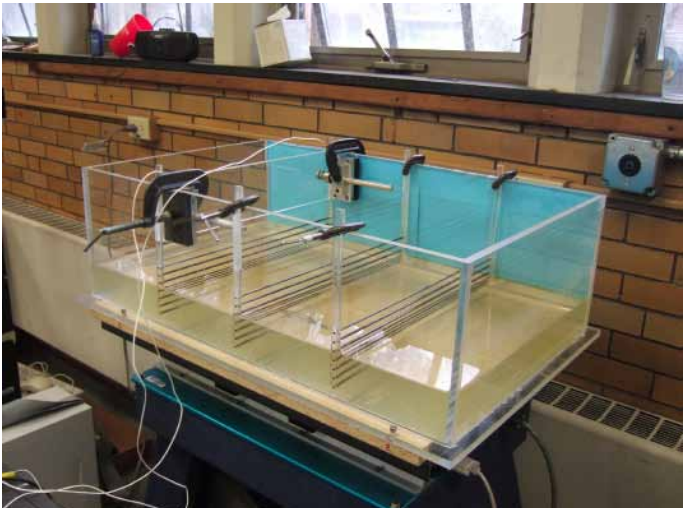
Figure 5. Experimental set up for screen force measurement on a shaking table (scale 1:10) (Source: Dae Kun Kwon)
