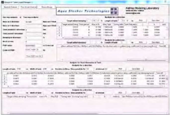
Figure 2. Aqua Sloshing Technologies: design portal for a tuned sloshing damper (Source: Deepak Kumar) 图2. 液体晃动技术：可调谐液体晃荡阻尼器设计软件（出自：Deepak Kumar）
