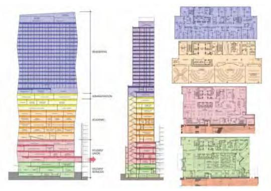
Figure 11. Section through Wabash Expansion, Roosevelt University, Chicago (Source VOA Associates Inc.) 图12. 罗斯福大学沃巴什扩建项目剖面, 芝加哥 (来源 VOA 事务所)
