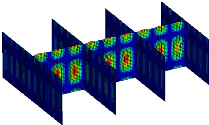
Fig. 10 Introduced imperfections between stiffeners at SPSWs
