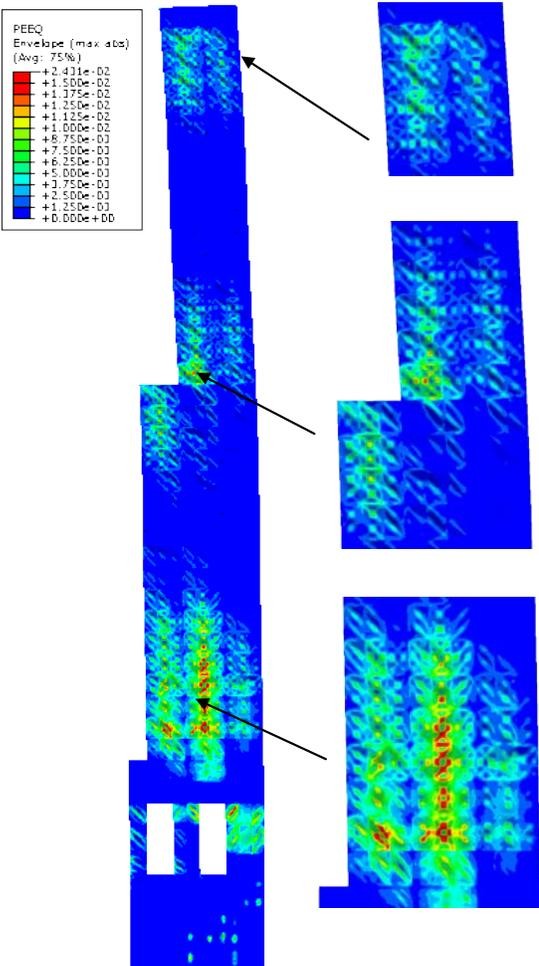
Fig.13 SPSW plastic buckling (tension field action)
