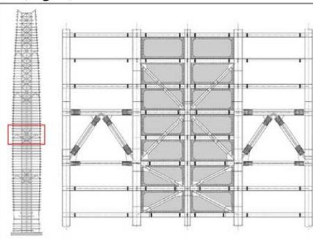
**Fig. 3.** Outrigger truss
