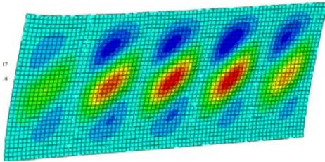
Fig. 7 Deformed SPSW shape
