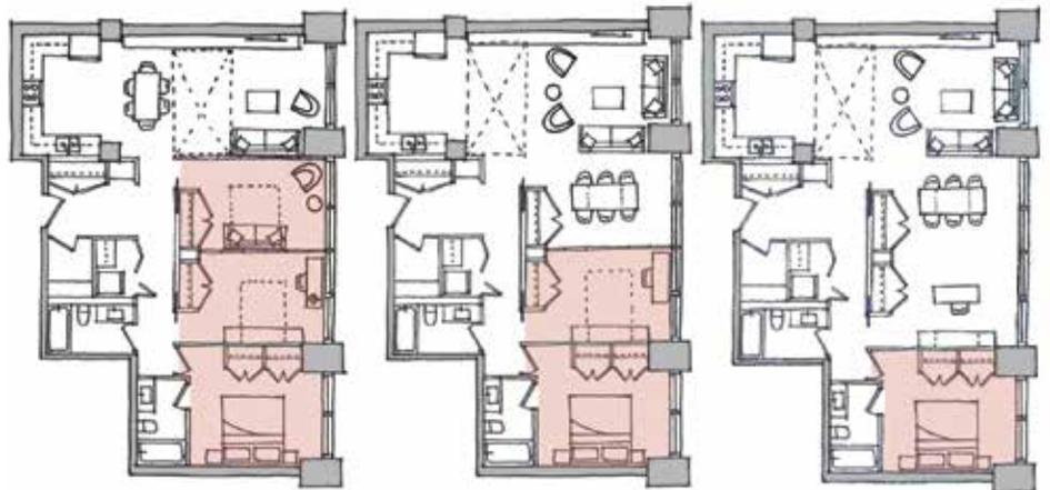
Figure 5. Examples of unit flexibility employing beam-and-column construction, folding and sliding partitions, and sliding pocket doors. Source: City of Toronto, 2017.
