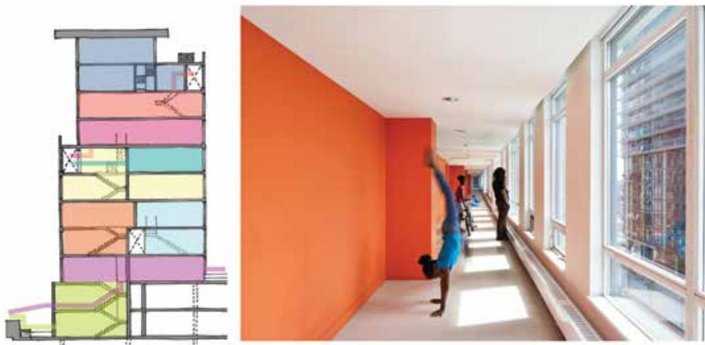
Figure 6. 150 Dan Leckie Way, Toronto – the multi-level “skip-stop” arrangement allows fewer and larger corridors, with finer attention paid to shared spaces. Source: City of Toronto, 2017.
