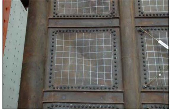
Figure 10. SPSW Panel after Test
