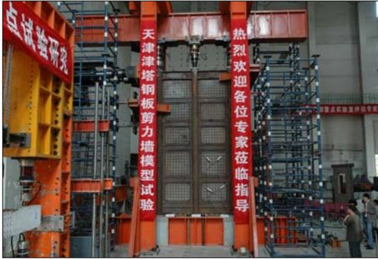
Figure 9. SPSW Assembly Test Set Up
