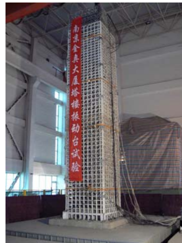
Fig. 14: Shake Table Testing
