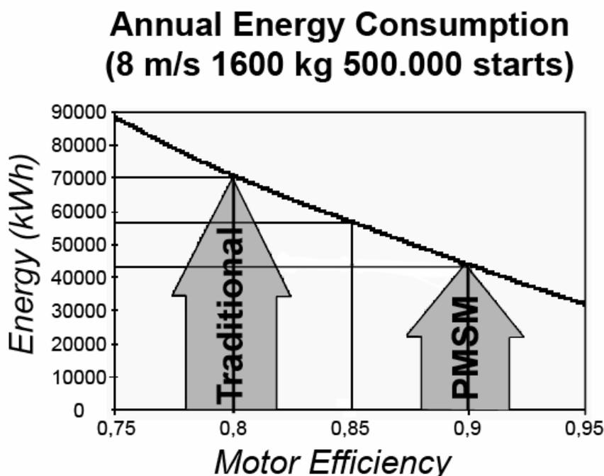
**Figure 7. Energy savings with EcoDisc® PMSM motors**
