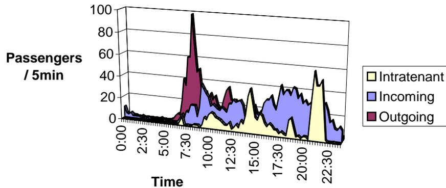
**Figure 2. Time slices for passenger generation in a one-tenant residential building.**
