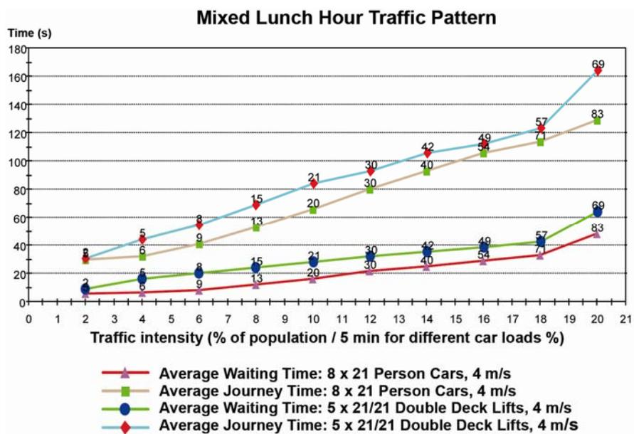
**Figure 3. Lunch Hour: Passenger waiting and journey times for eight conventional single deck elevators, and five double deck elevators with the same deck size**
