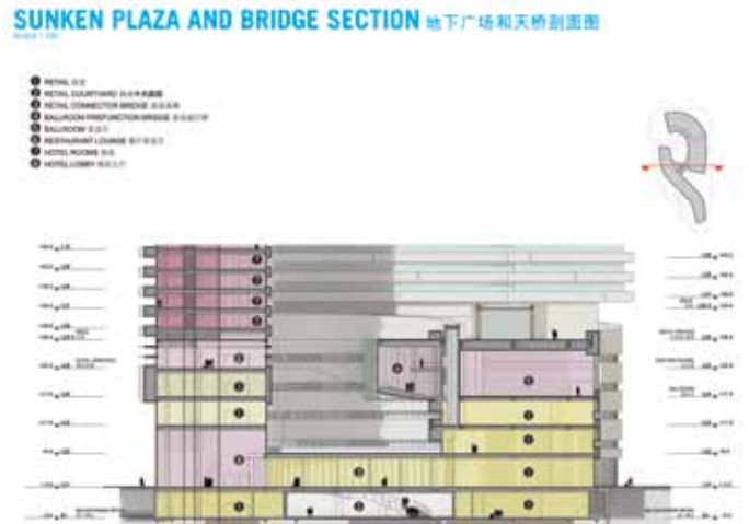
Figure 2. Xiamen Eton Center, section through pedestrian bridges. (Source: NBBJ) 图2. 厦门裕景中心，穿过步行桥的剖面图（出自：NBBJ）
