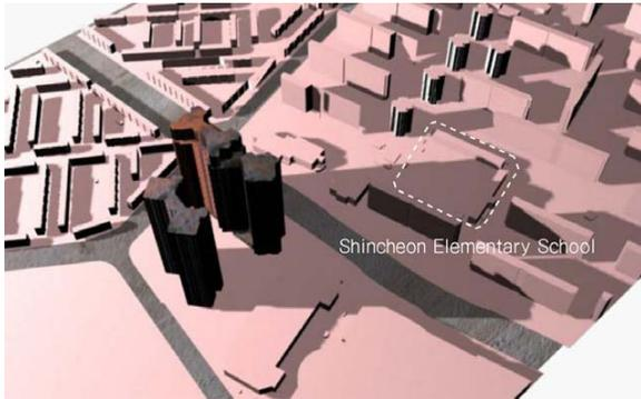
Fig. 6. Sunlight Access Simulation of Jamsil Galleria Place
