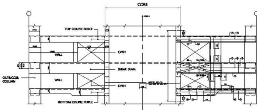
Figure 6 Outrigger Elevation.
