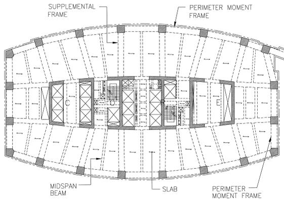
**Figure 10** Typical Framing Plan.
