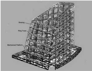
**Figure 11** Isometric Lantern.
