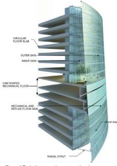
Figure 6. Typical zone section perspective view
