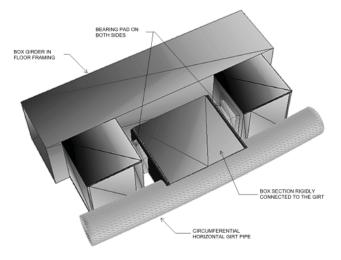
Curtain wall thrust block detail
