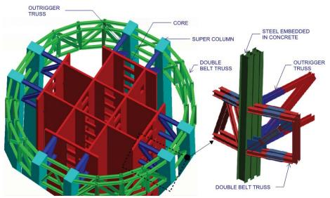
Figure 5. Mega frame for Shanghai Tower and outrigger detail
