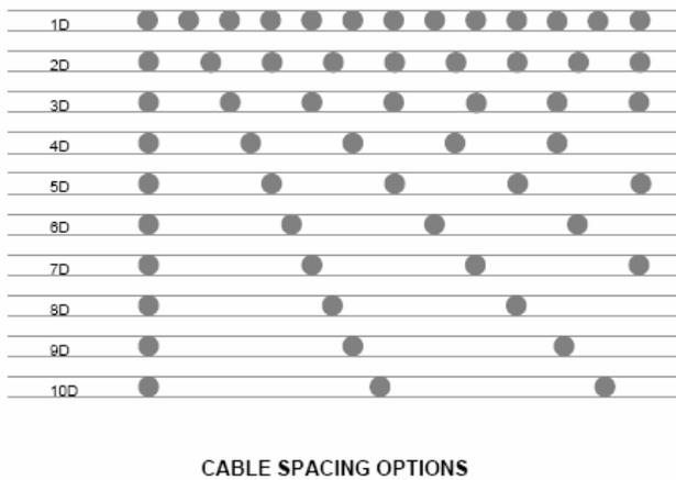
Figure 14. Diagrams showing the spacing between cables based on the cable diameter.
