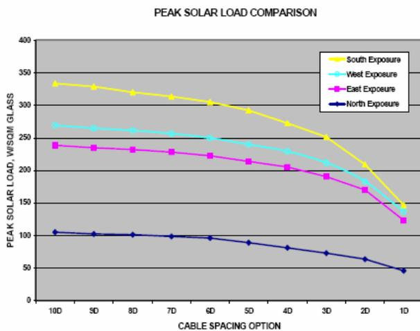
Figure 15. Reduction in peak solar cooling load based on cable spacing and facade orientation.
