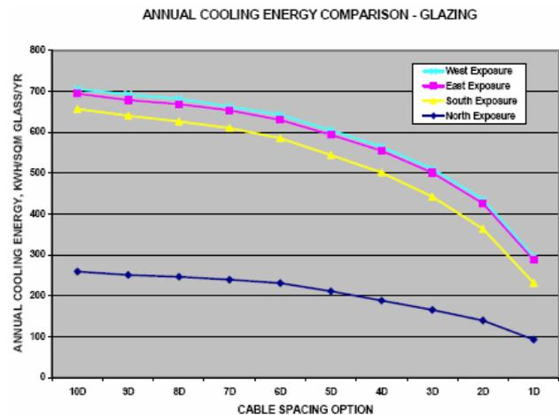
Figure 16 Reduction in peak solar cooling energy based on cable spacing and facade orientation.
