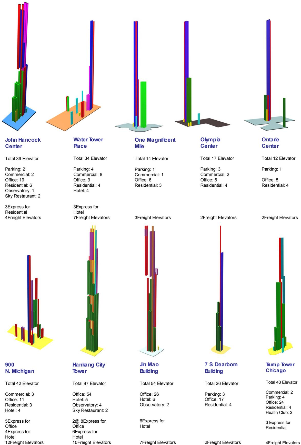
**Fig. 6.** Analysis of Elevators – Passenger / Freight / Express Shuttle
