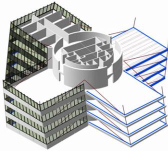
**3d.** Isometric drawing of cylindrical core
