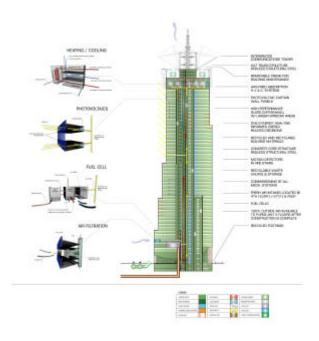
Fig.1. Sustainable Components of Four Times Square
