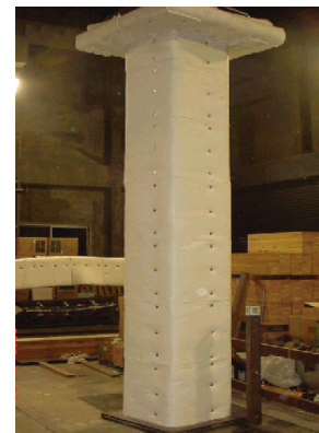
Photo 1. Blanket-type Fire Protection
