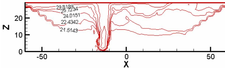
Fig. 6-2. Distribution of temperature in smoking shaft at 480s
