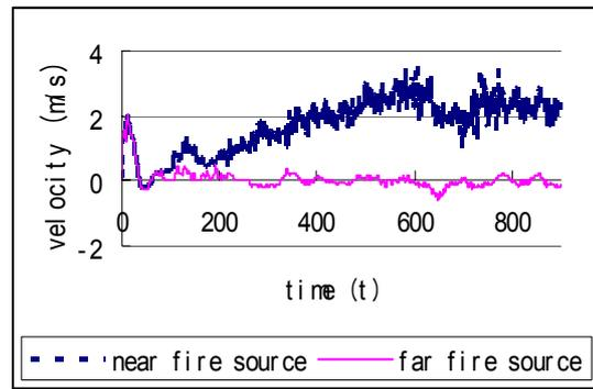
**Fig. 4-2.** flow velocity versus time in smoking shaft system with 200,000m<sup>3</sup>/h mechanical air supply and high HRR
