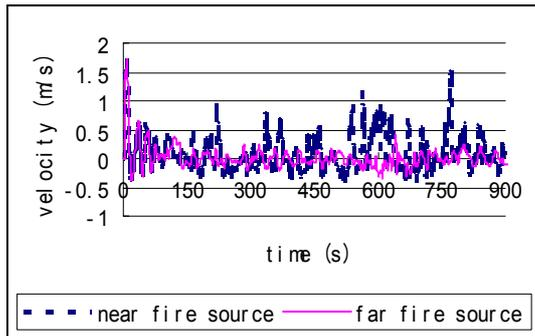
**Fig. 2.** flow velocity versus time in natural ventilation system
