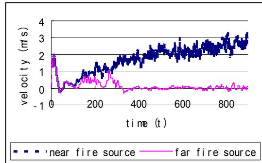
**Fig. 3.** flow velocity versus time in smoking shaft system with low HRR
