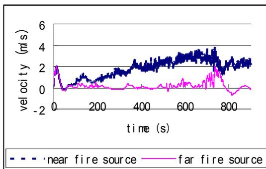
**Fig. 4-3.** flow velocity versus time in natural ventilation with 900,000m<sup>3</sup>/h mechanical air supply and high HRR
