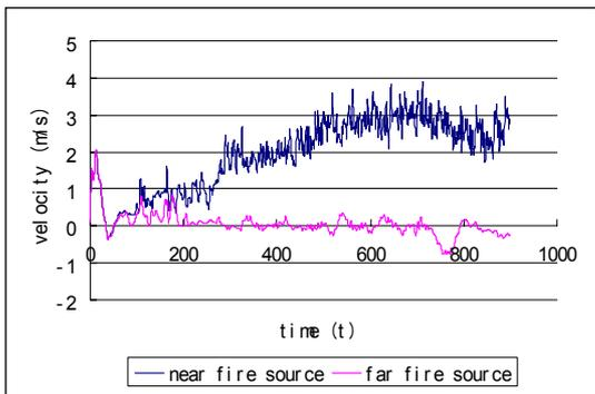
**Fig. 4-1.** flow velocity versus time in smoking shaft system with high HRR
