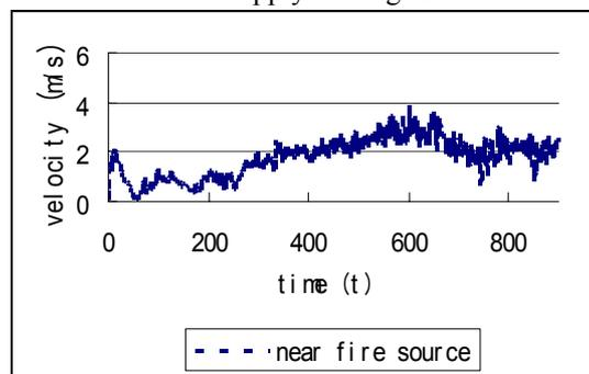
**Fig. 5.** flow velocity versus time in partial smoking shaft which are near the fire source when far smoking shafts are closed
