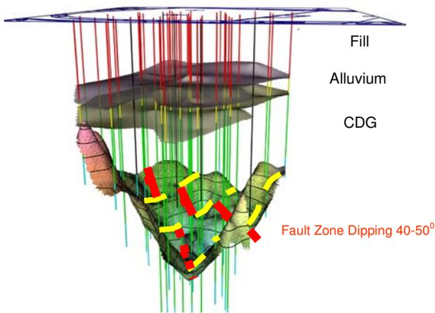
Fig.6. The 3D inferred rockhead contour
