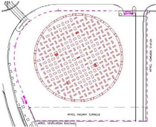
Fig. 7. The Piling Layout Plan
