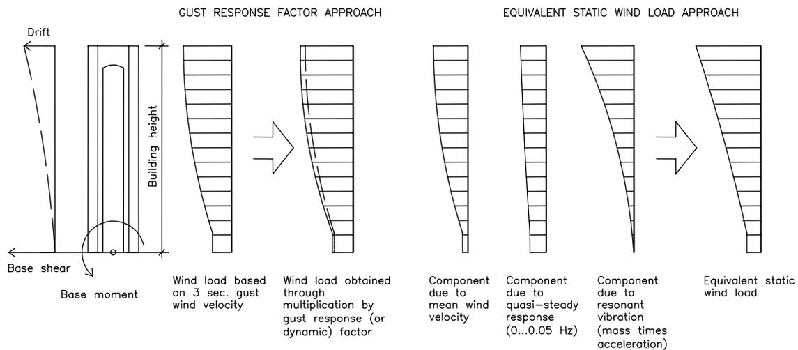
Fig. 2: Comparison of typical design code approach vs. equivalent static wind load approach.
