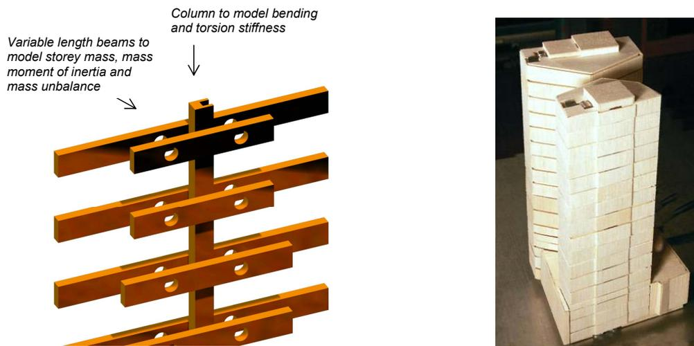
*Fig. 3: Proposed spine-cladding system for aeroelastic model of tall building; 1:500 model for the Tallinn Tornimäe Twin Tower by the author.*
