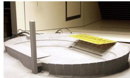
Fig. 6: a) New roof structure of the Helsinki Olympic Stadium (photo K2S Architects Ltd) and b) aeroelastic wind tunnel model (photo by the author).
