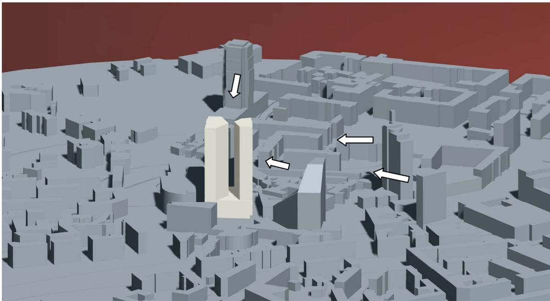
*Fig. 1: Wake buffeting issue as illustrated in the context of the Tornimäe Twin Tower laying among sparsely built tall buildings in Tallinn, Estonia. Arrows are indicating possible problematic wind directions for the new building.*
