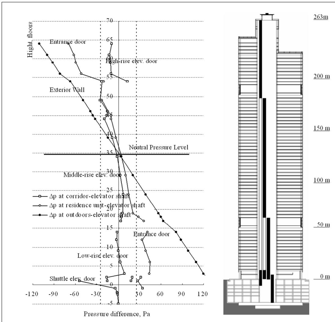
Fig. 12. Field measurement results of building B
