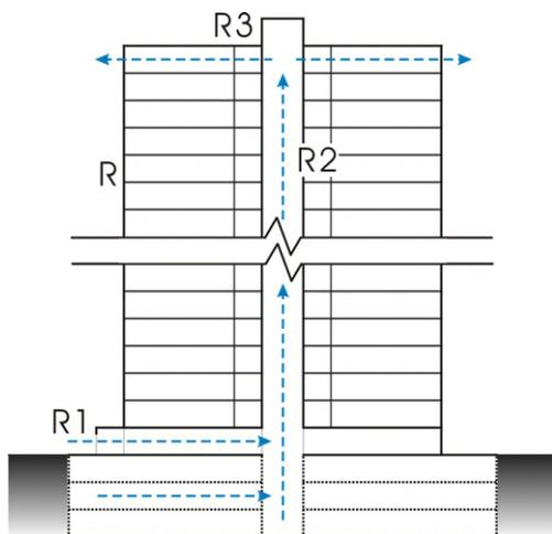
**Fig. 4.** Diagram of airflow path due to stack effect
