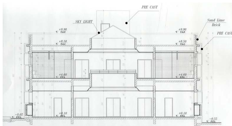
Figure 3: Cross section in a classroom wing
