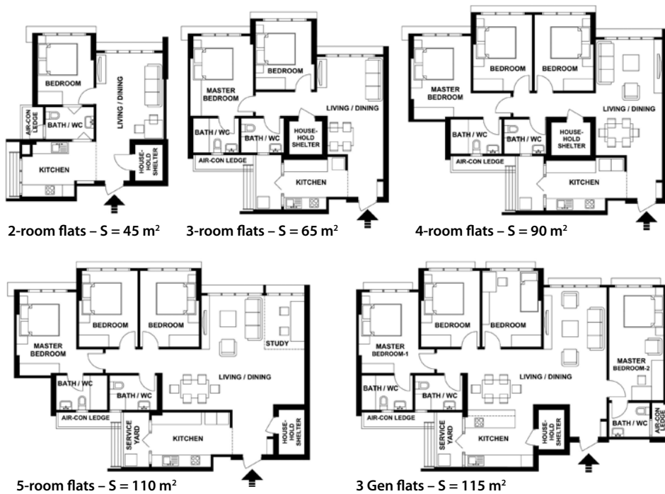
Figure 15. Basic types of HDB flats: two-room flats, three-room flats, four-room flats, five-room flats, and 3Gen flats.
