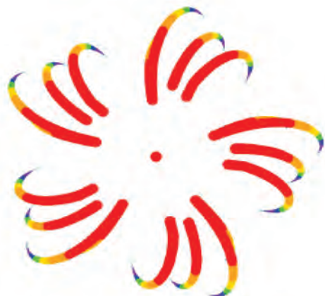
Figure 11. Elastic rotation of Tower columns under self weight (Source: Peyman Askarinejad) 图11 自重工况下的大楼弹性旋转(资料来源: Peyman Askarinejad)
