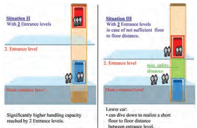
Figure 3. Flexibility of the TWIN-System with 2 cars in one shaft on floor distances
