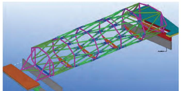
Figure 3. Structural steel framing general arrangement (source AGC-A)
