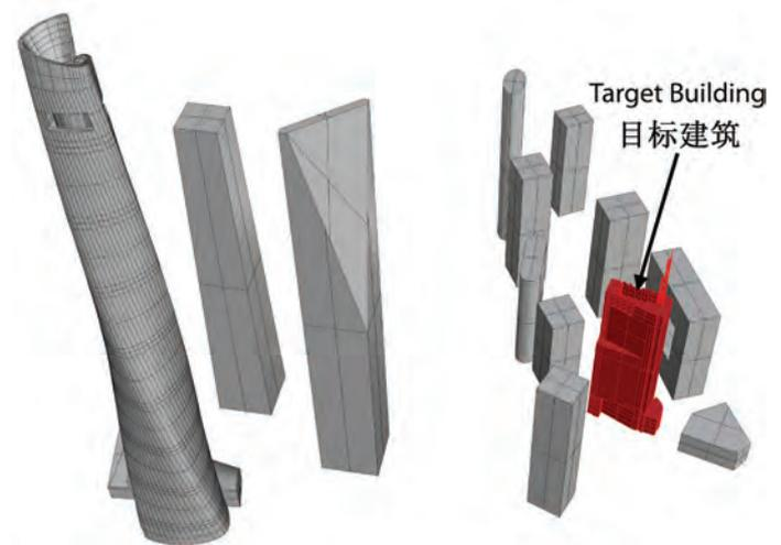
Figure 1. The numerical wind tunnel models
