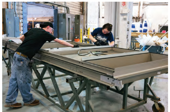
Figure 3. CW unit frames are factory assembled from fabricated aluminum extrusions and gaskets fitted to extruded raceways (Source: Mic Patterson). 图三: 工厂组装的幕墙单元体 (来源: Mic Patterson)
