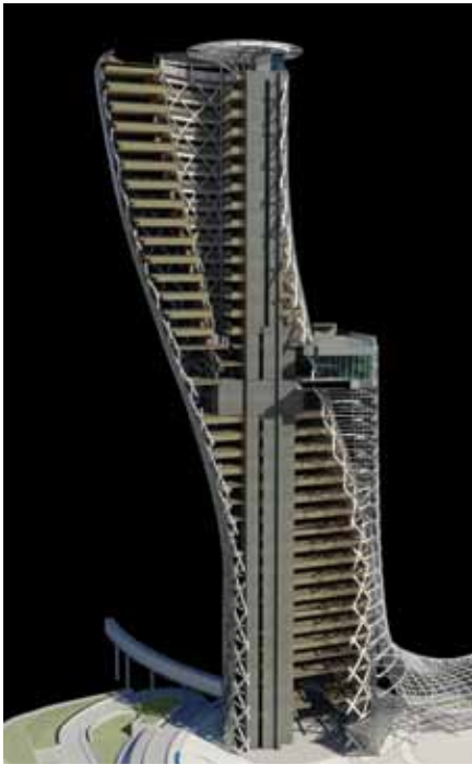
Figure 6. Model section showing the funnel-shaped atrium © Jeff Schofield
