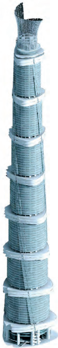
Figure 3.1. With the outer skin removed, the regular circular floor plates are revealed. (Source: Gensler)
