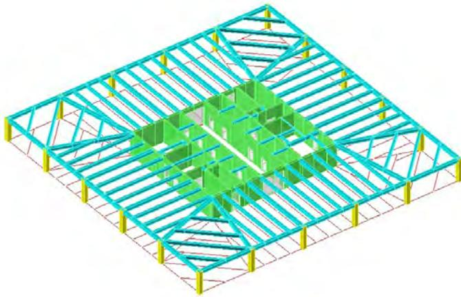
Figure 3.49. Floor systems layout optimization – Optimization design scheme (Source: Xin Zhao)
