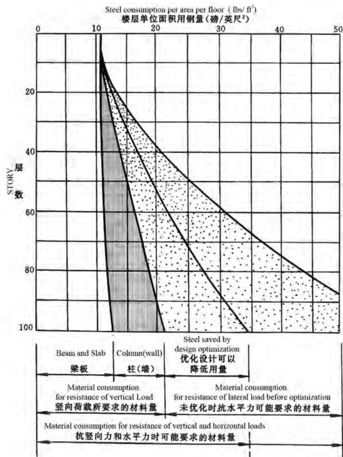
Figure 3.48. The change of structural cost with structural height (Source: Lin T.Y. & Stotesbury, S.D.)
