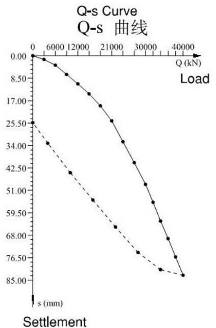
Figure 3.8. Test Pile: load-settlement curve (Source: Shanghai Jianke Technical Assessment of Construction, Co., Ltd)
