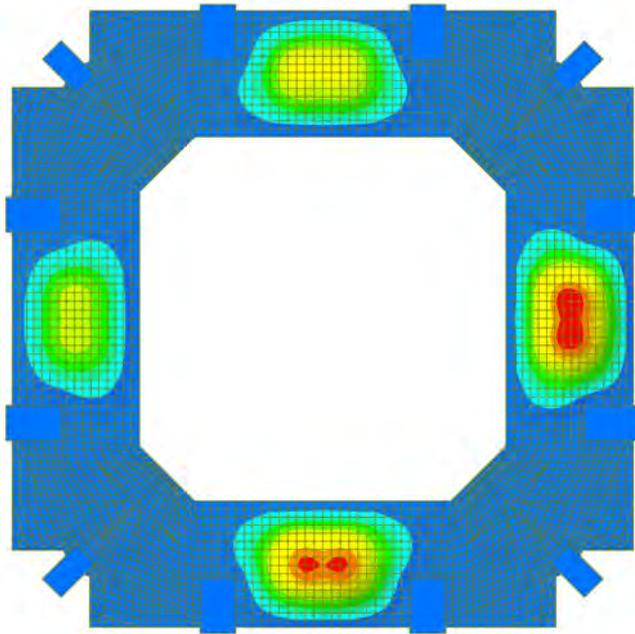
Figure 3.10. First Mode Shape of Floor Vibration (Source: Thornton Tomasetti)
