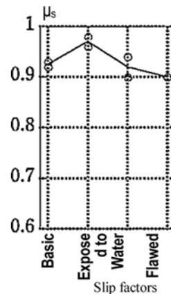
Figure 22. Relations between construction troubles and slip factors.
