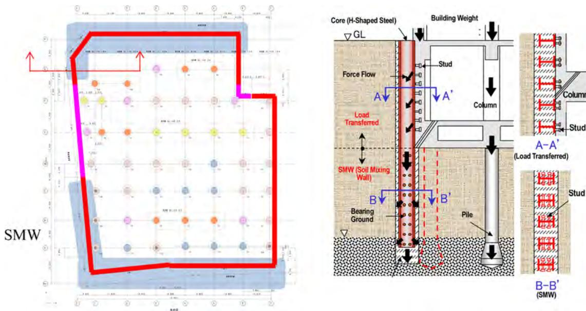
Figure 12. Pile plan (left) and sectional view of SMW (right).
