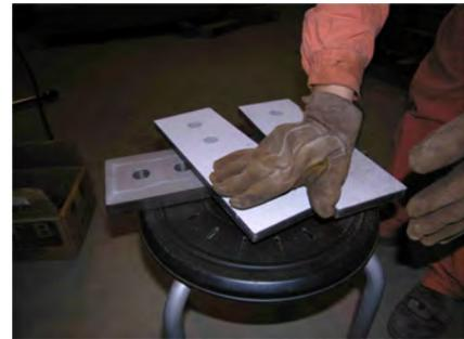
Figure 25. Oil-stained test: Oil-stained leather glove.
