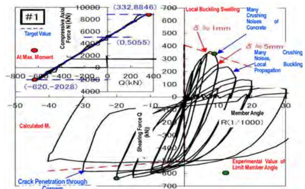
Figure 16. Load-deformation relations.
