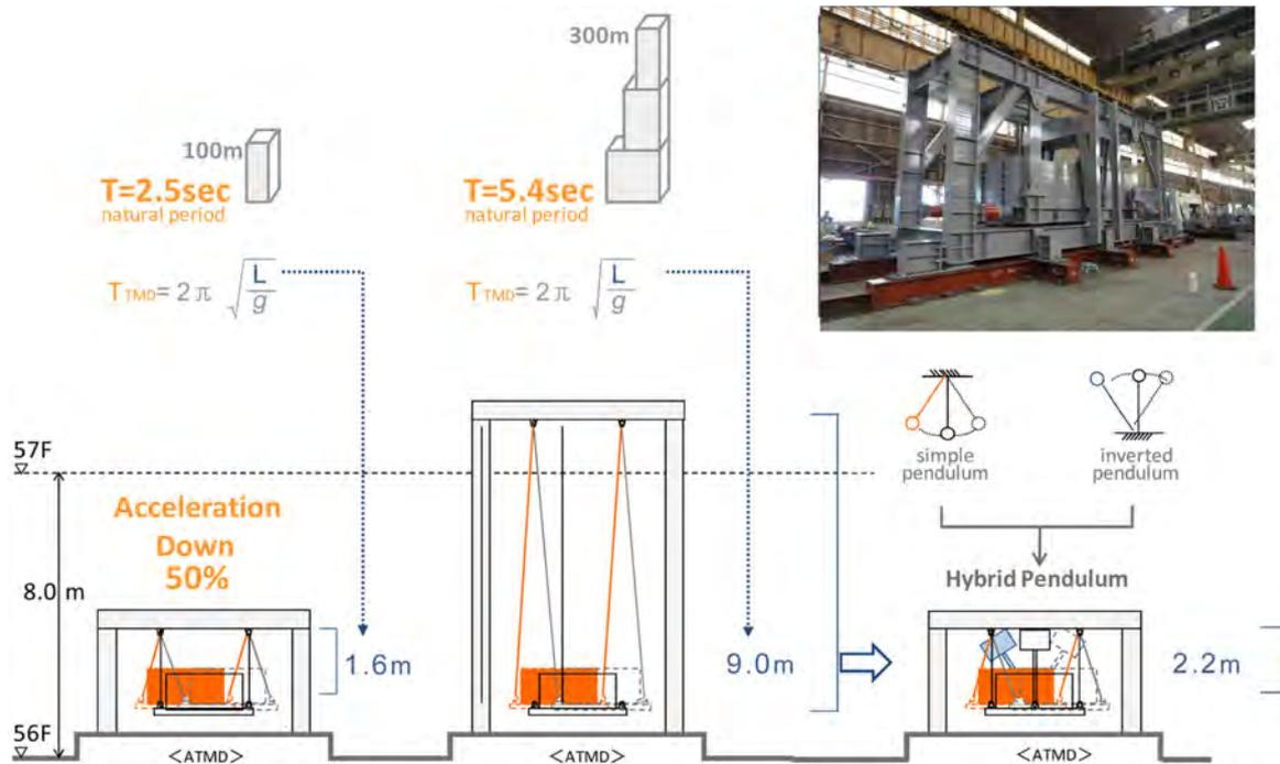
Figure 33. Illustration overview of hybrid pendulum ATMD.
