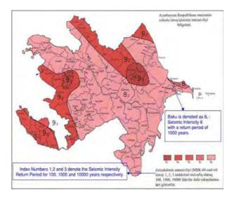
Figure 6. Seismic Intensity Zones of Azerbaijan (AZN10).
