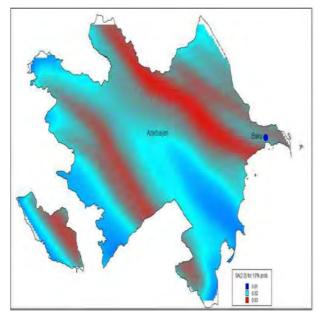
Figure 5. Spectral Acceleration for P = 2.0 sec with a Return period of 475 years by Akhundov et al. (2011).
