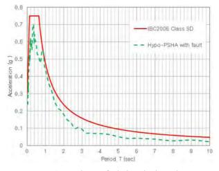
Figure 10. Comparison of design horizontal response spectra with fault underneath the Site.
