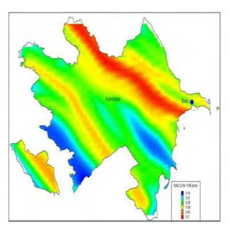
Figure 3. Spectral Acceleration for P = 0.2 sec with a Return period of 475 years by Akhundov et al. (2011).
