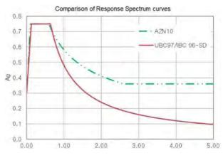
Figure 7. Comparison of Response Spectrum Curves, (AZN vs UBC/IBC).
