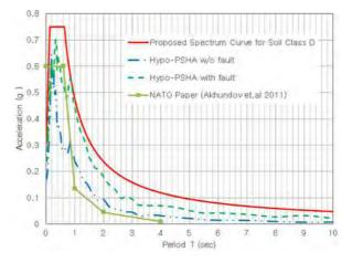
Figure 11. Comparison of Response Spectra.
