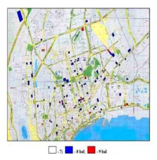
**Figure 1.** Seismic Zoning Areas in Baku City (NATO Science for Peace and Security Programme by Akhundov et al. (2011).
