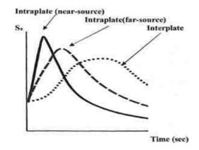
Figure 8. Comparison of Inter and Intra-Plate Earthquakes by Gioncu, Mazzolani (2011).
