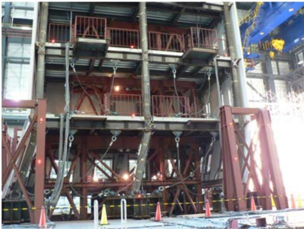
**Figure 6.** Story collapse mechanism caused by local buckling in the first-story column observed by experiment.
