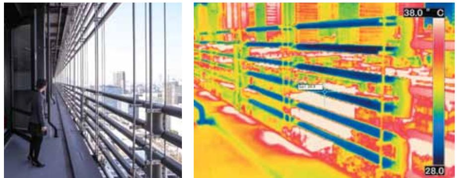
Figure 13. Thermographic photo of NBF Osaki Building's façade after the BioSkin was activated. © Gankosha
