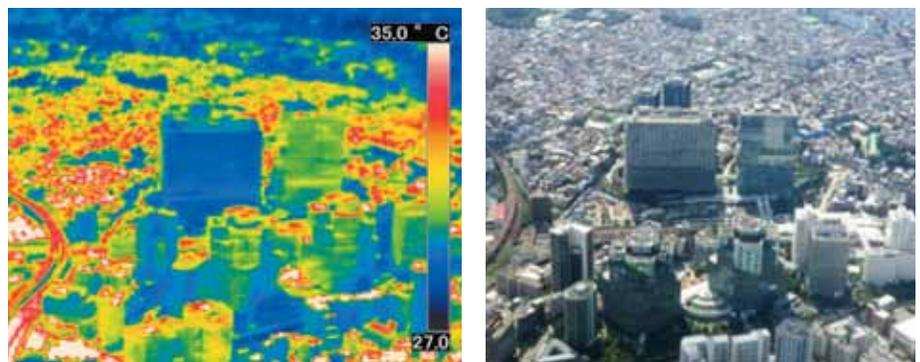
Figure 14. Aerial thermographic photo of the BioSkin-clad building. © Nikken Sekkei
