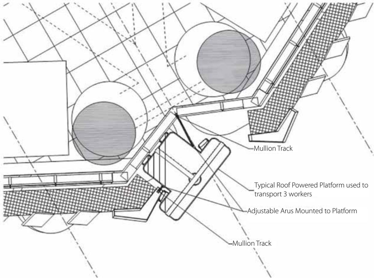
designed to provide safe and efficient access for glass replacement. Introducing the catwalk as one of the major façade elements contributes toward the increase of the cleaning cycle frequency from 4 times per annum to 15 times per annum, which is calculated with three BMU's on the roof with capacity for three workers per platform.
