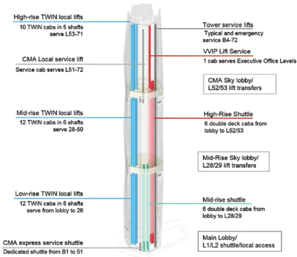
Opposite: Elevator system configuration showing use of double deck and TWIN cabs. Source: HOK
