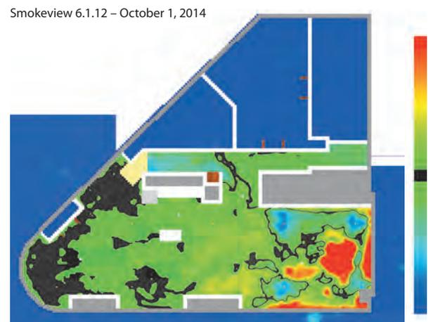
Figure 9. Temperature in Level 33 shortly after sprinkler activation. Red shows high temperatures (100°C or more), blue shows low temperature (20–35°C).
