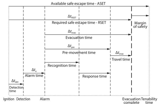
Figure 4. Example of a timeline comparison of the Available Safe Egress Time (ASET) and Required Safe Egress Time (RSET). Source: PD 7974-6:2004.
