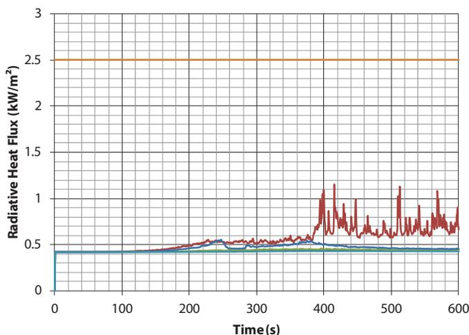
Figure 8. Radiative Heat Flux received from smoke during means of escape phase.
