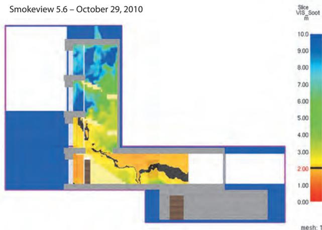
Figure 7. The visibility at 243 seconds in the upper stair. Blue shows good visibility (10 meters), red shows bad (0 meters).
